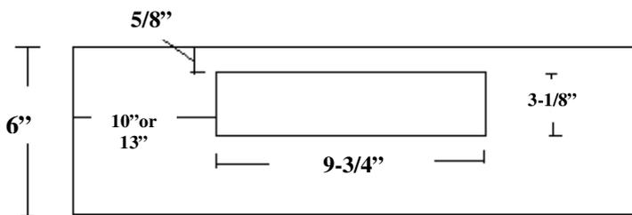
Use 3-1/4 x 10" or larger size of ducting. Do not reduce size; make all turns gradual, no short corners. If run longer than 10 ft., enlarge duct after first 10 ft. Tape all joints for tight seal. .
